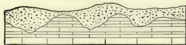
FIG. 185.—Diagram to illustrate variation of drift thickness due to buried hills and valleys.
